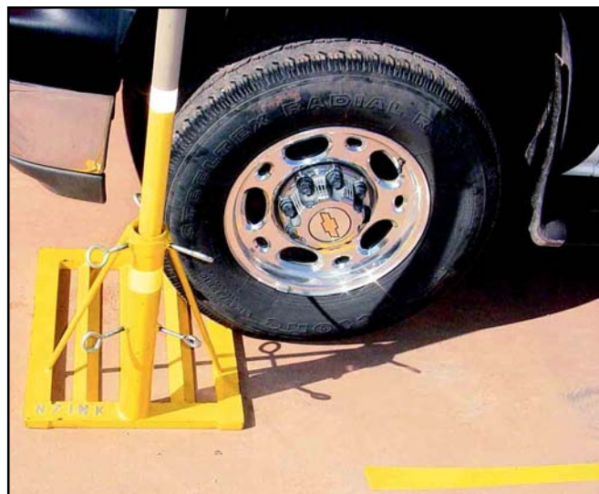
Figure 4—The RORO (“big foot”) mount. This was custom-built for the author by a welding shop (see text).
