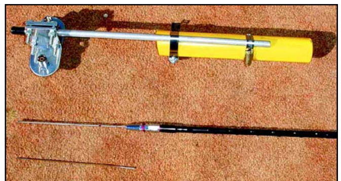
Figure 2—A coat hanger is used as a prototype "stinger" during testing and requires that the paint be scraped off its end. It is shown next to a new stainless steel tip. The dipole adapter is shown at the top.
