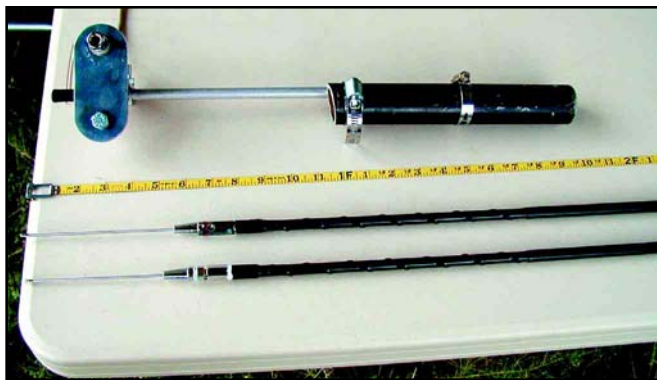
Figure 3—A top view of the assembled dipole adapter used to mount and secure both antennas, which are shown below it.
